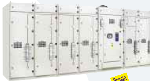
Dual Feed, 4 Motor Multistart 6600V, 250A, with disconnect switch for each line input and motor output
