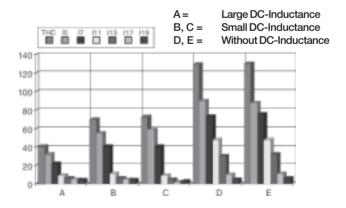
Figure 7.10. Harmonic current with different DC-Inductances.
