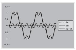
Figure 2.3 The total current as the sum of the fundamental and 5th harmonic.
