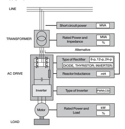
Figure 7.1 Drive system features affecting harmonics.
