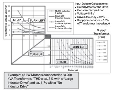
Figure 7.9 Total harmonic distortion nomogram.
