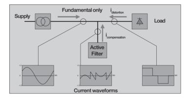
Figure 8.3 External active filter principle diagram.
