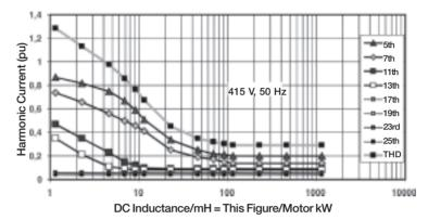
Figure 7.7 Harmonic current as function of DC inductance.
