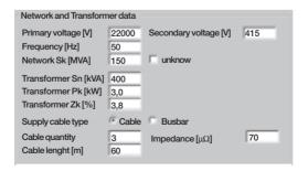
Figure 4.6. The network and transformer data input is given here. For standard ABB transformers the data is shown automatically.
