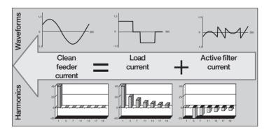
Figure 8.4 External active filter waveforms and harmonics.
