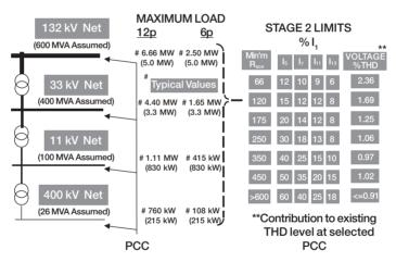
Figure 5.1 Limits on Harmonics in the proposed EN61000-3-4.
