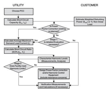
Figure 6.1 Evaluation of harmonic distortion.
